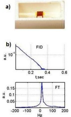
**Fig.2:** a) Probe Solenoid; b) Probe FID and FT
